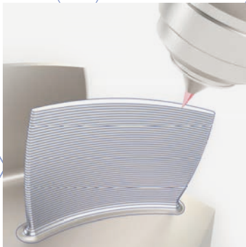
Additive Manufacturing of a Blisk
